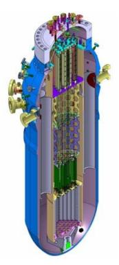
Fig. 1. Reactor Pressure Vessel
