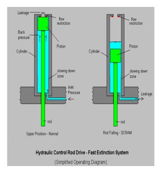
Fig. 5. Simplified operating diagram of a hydraulic control rod drive (Fast Shutdown System)
