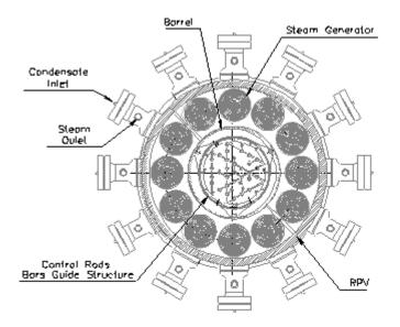
Fig. 4. Steam Generation lay out
